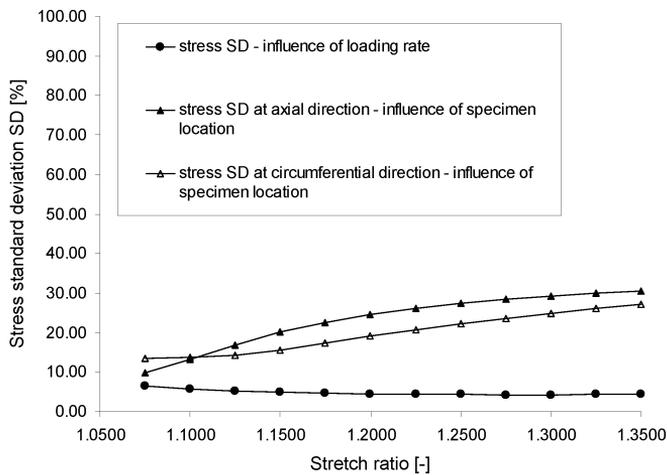
Fig.11: Standard deviations [%] in stresses as function of stretch ratio [-]
