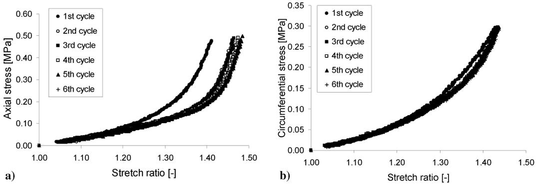
Fig.9: Cyclic stress-stretch responses during uniaxial tension test
