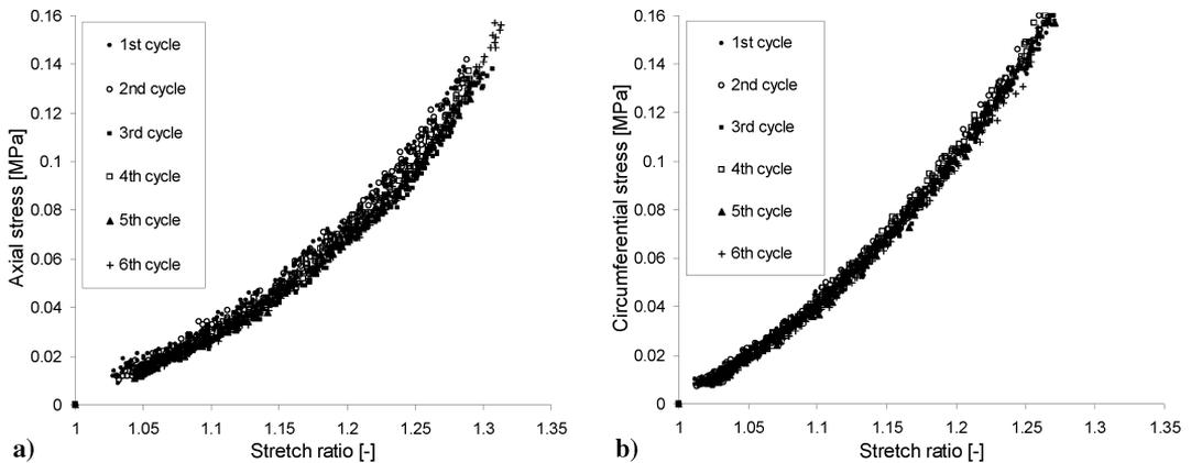
Fig.7: Cyclic stress-stretch responses in equibiaxial tension tests
