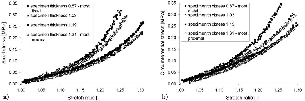
Fig.10: Equibiaxial stress-stretch responses in various locations along the thoracic aorta; a) axial direction; b) circumferential direction
