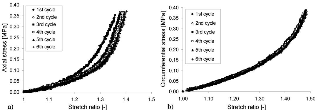
Fig.8: Cyclic stress-stretch responses in planar tension tests
