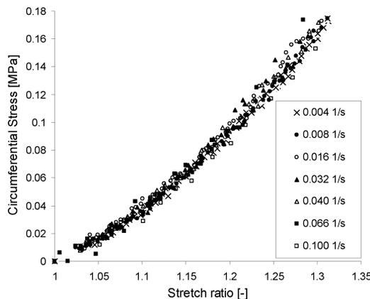
Fig.6: Equibiaxial stress-stretch responses for different loading rates
