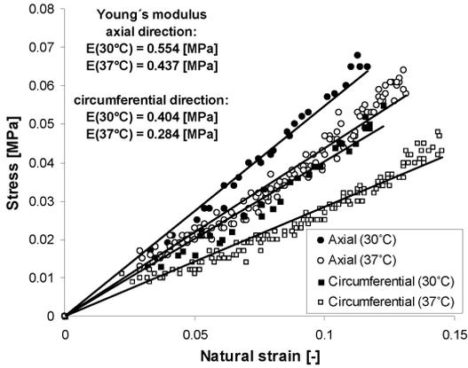
Fig.4: Equibiaxial stress-natural strain responses for different temperatures
