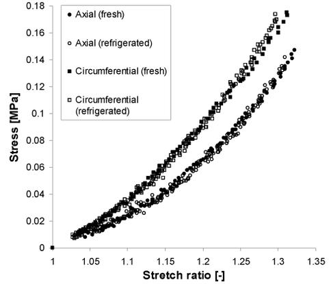
Fig.5: Equibiaxial stress-stretch responses for fresh and refrigerated specimen
